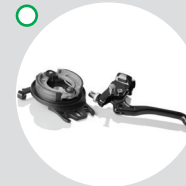
Hub brakes Available on all wheels sizes. Needs extended handles option.
