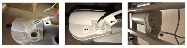
Please be sure to connect the corresponding number to the number on each actuator. Backrest (connected to the control box) = 1, Knee break = 3 and the two Hi-Lo actuators in the head and footboards = 2 & 4. Push the connector fully into the actuator and push in the locking clip until it clicks.
