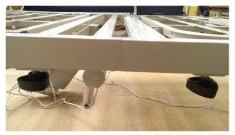
Unscrew the 4 hand screws on both the head and foot halves of the frame. Use the bars provided to connect the two halves of the frame together, ensuring the end of each bar with the blue dot is inserted first into the fame with the blue dots. Also note the location tab should be facing down as shown in the photo above. Once the two halves of the frame are fully pushed together, hand tighten the hand screws.
