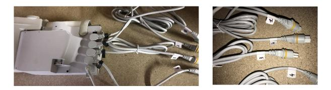
The main control unit and the back and foot rest actuators should already be attached to the bed frame (shown above detached). The cables will also be attached to the control box with the connectors for each actuator numbered up 1 - 4.
